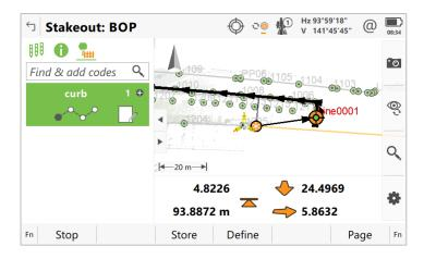
With this extension of the **Stake points** and **Stake to line** apps, measure and check routines can now be done in the same app while using the full coding functionality. This enables staked/checked data to be used to create an entirely new data model, which can then be compared to the original design model.
