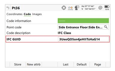
This will allow content within a Captivate job to be associated with the IFC object they originate from and make it possible to use and correctly associate this data throughout the lifetime of the IFC data.
