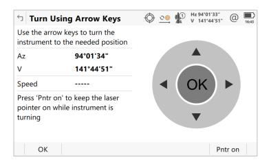
Press **Pntr on (F6)** in the **Turn Using Arrow Keys** panel to use the laser pointer while positioning the instrument. The **Pntr auto (F6)** button allows returning to automatically switching the laser pointer off while turning the instrument.
