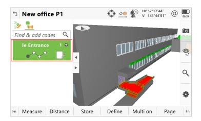
Once the points are imported into the office software, the code and attribute allow automatically matching the measured points to the relevant IFC object. This saves time, eliminates the need for manually matching measured points to IFC objects and makes this process less error prone.
