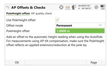
With Leica Captivate v7.50 it is possible to configure the length of a pole extension and apply it automatically to each AP20 measured pole height change. This way, even when working with an extension to the AutoPole, automatic height measurements can be used as a guarantee to always apply the correct pole height.
