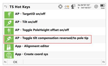
With Leica Captivate v7.50 there is a new hotkey to allow toggling between the two tilt compensation modes without leaving the app. When tilt compensation is off, pressing this hotkey turns tilt compensation on and switches the tilt compensation mode at the same time. A message indicates the change of tilt compensation modes.
