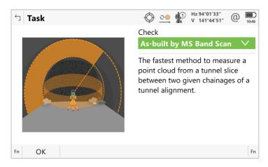
The new method allows for a much-improved work speed and is also more flexible when scanning a tunnel profile by not making it necessary to move an already set up instrument outside the defined chainages.
