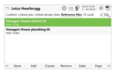
Previous versions of Captivate would allow only one IFC file to be viewed at a time. With Leica Captivate v7.50 it is possible to display the information from multiple IFC files simultaneously, giving a more holistic view of the available design elements in a project.
