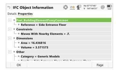
This new feature allows for object specific information, such as geometry, properties, or materials to be available in the field and seen directly on site as needed.
