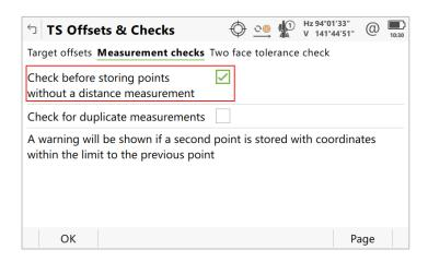
The new check can be found in the **Point storage** settings, within the **TS offsets and checks** panel. Note that per default, the check box will be activated, meaning warning messages will be shown for angle only measurements unless the check box is being deactivated.
