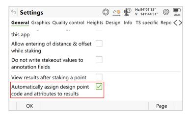
Note that per default the new setting is active in the **Stake points** and **Stake to line** apps while it is deactivated in the **Measure to line** app. When activated in the Measure to line app, the coding and linework tab will not be shown in the app as codes are applied automatically.
