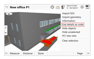
For each point measure afterwards, the IFC object name will then automatically be stored as the code for the measured points and the GUID will be written as the value for attribute 1 of that code.
