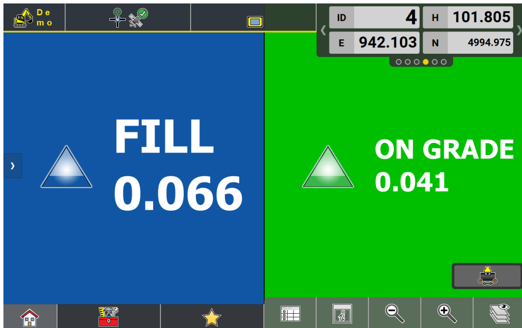
Full screen view showing Left and Right bucket edges Cut/Fill information.
