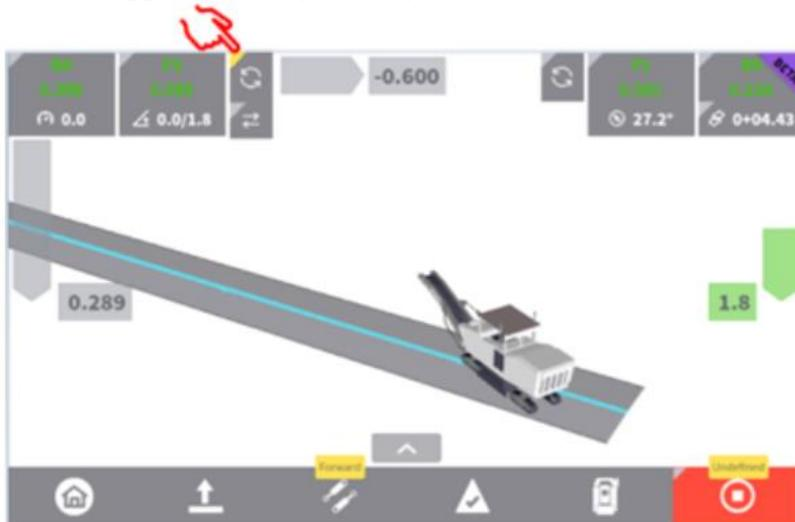
By using the Toggle button, the Spares F3 and F2 will change their position and F2 will become the Active spare for the Primary Mast
