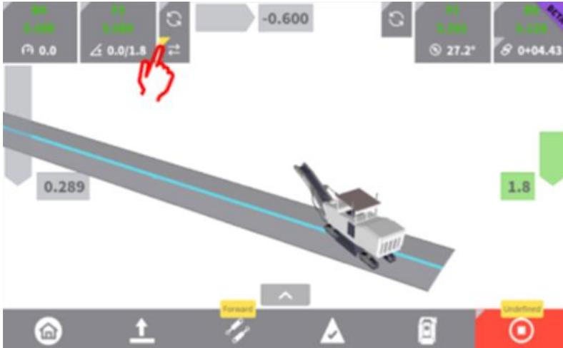
By using the Toggle button, the Spares F3 and F1 will be reassigned; F1 will become active spare for Primary mast and F3 active spare for the Secondary mast.
