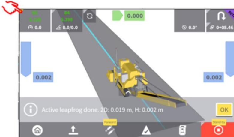
Manual leap with a **TAP&HOLD** on the Active / Primary/ Secondary mast.
