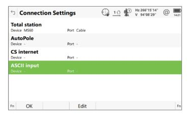
To follow the current serial interface standards to be able to still receive the information from the external device, Leica Captivate running in Windows tablets, needs to be configured by defining a format for the incoming messages.
