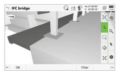
From Leica Captivate v8.50 onwards, the minimum zoom distance limitation has been decreased, which allows zooming in much closer to objects. This means that objects can be viewed in more detail, which also makes selecting small or complex objects much easier. The image below shows that the base of the pillar can be zoomed in too much closer than previously.
