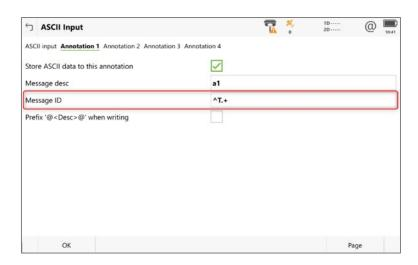
In the above example, all messages starting with "T" are displayed in Annotation 1 field. The following are some real examples of received data:
