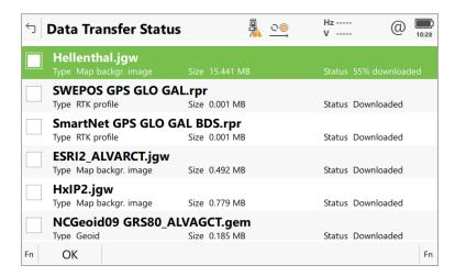
The **Regional configurator** tool supports and recognises all types of Leica Captivate objects, and automatically places the downloaded objects into the correct location, so that Captivate can directly use them without any further steps required.
