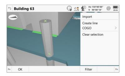
Points created with the snapping tool will automatically have the reference data layer information assigned to the Point code, and for IFC data, include the GUID as an annotation.
