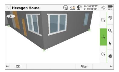
**Snap to arc/circle centre point** – allows snapping to the centre point of an arc or the centre point of a circle. This makes it easy to create individual points at the centre of circular objects such as the centre of a column within an IFC file.
