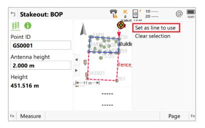
This new option ensures that when needing to change the reference line, the ongoing field task is not interrupted by avoiding the need to change panels or stop the measurement process.
