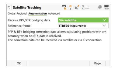
This new PPP reference frame database will be included by default in all new field controllers being delivered with Captivate v8.50.
