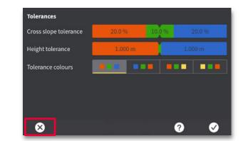
**Step 6:** Use the +/- buttons to increase or decrease the tolerance for each field (**fill**, **on grade** and **cut**). Press X (exit).
