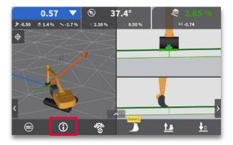
**Step 1:** Turn your machine so the boom points toward the desired direction of X, then press the "set X-direction" button.
