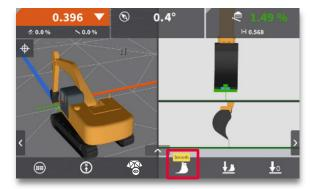
• The new bucket will be automatically applied, and its name will be visible above the bucket icon in the quick access bar.
