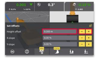
**Step 2:** Use +/- to toggle height offset, or press the value field to enter a value.
