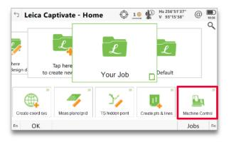
**Step 1:** When your total station is set up, enter the "Machine Control" app. Make sure it is installed, and that you have the corresponding license (<u>Workflow</u> <u>11.4.</u>).
