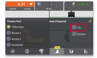
**Step 2:** Press the "Tilt" box in the "Auto Prepared" section.
