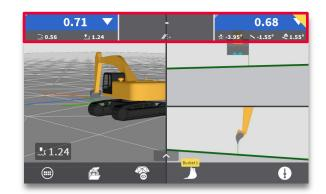
• The run-screen indicators update to current selection (The 3D option "Bucket left height, direction, bucket right height" is shown here).
