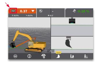
**Step 5:** Press the "PREP" button to activate CoPilot prepared mode (can be configured to an external button).
