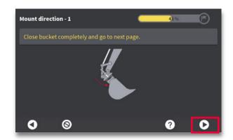
**Step 6:** Close the bucket completely and press right arrow (next).
