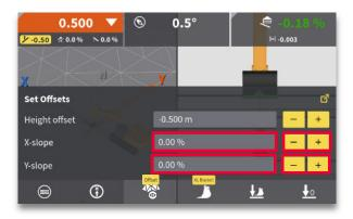
**Step 2:** Use +/- to toggle X- or Y-slope, or press the value field to enter a value.
