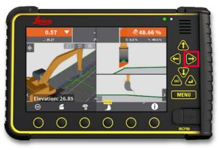
**Step 2:** Press **right** hard key to toggle height tool point to middle position.
