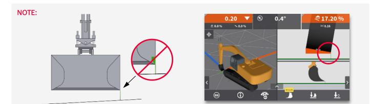
The typical green arrow indicating the height tool point will not be shown when "closest to" height tool point has been selected. The green line will still appear, and change position depending on what tool point is closest to the design.
