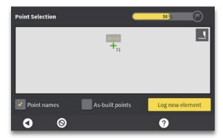
**Step 6:** T1 is assigned to the first point. Repeat steps 4-5 for the remaining points in the desired baseline.
