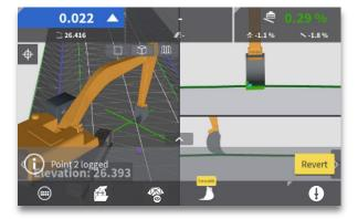
**Step 5:** If necessary, press "Revert" to remove previously logged point.
