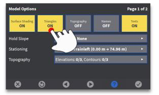
**Step 3:** Features with additional explanations offered are framed in blue. Press a blue framed feature to view its associated help screen. "Triangles" shown here.
