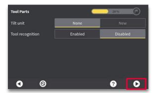
**Step 5:** Select "tilt unit" and "tool recognition" (if applicable). Press right arrow (next).
