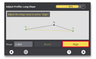
**Step 15:** Press "Align" to align your long slope to the entered value beginning at the point we adjusted in step 8.
