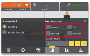
**Step 2:** Press the boxes for the functions that should be controlled automatically.
