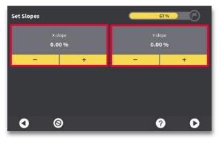
Step 7: Set X-slope and Y-slope to desired values.
