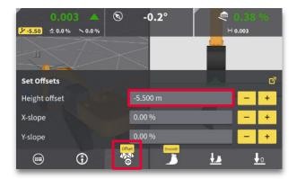
**Step 5:** Verify applied offset value. Press the model options menu to return to run-screen.
