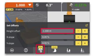
**Step 4:** Verify applied offset. Press the model options menu to return to run-screen.
