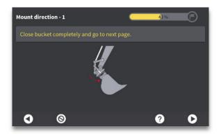
**Step 14:** Open or close the bucket so tip of bucket is vertically aligned with bucket pivot point. Use a plummet, or carpenter's level, to verify angle.
