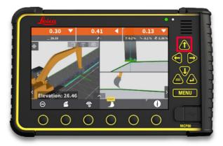
**Step 3:** Press **up** hard key to toggle side tool point to right tip position.
