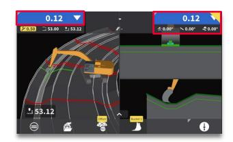
• Cut/fill values will be shown, providing guidance to new height offset. Original grade will still be shown in cross-section with applied offset.
