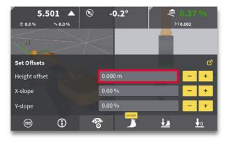
**Step 3:** Enter height offset values into the panel (press + or – ). On-screen surface illustrations, and dig value, updates to reflect entered height offset.
