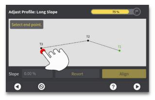
**Step 12:** Select end of baseline long slope by tapping the desired point.
