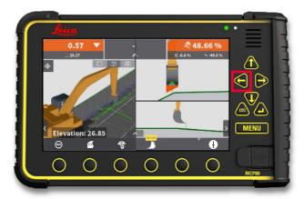
**Step 4:** Press **left** hard key to toggle height tool point in opposite direction.
