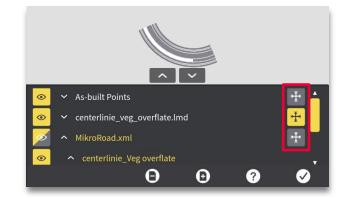
Step 3: Select which models you want to make referential in the run screen. NOTE: models cannot be made referential in the run screen if visibility is turned OFF (Step 2).
