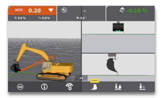
**Step 6:** Place bucket inside model boundaries, and within operational height window (which is 30cm.)
