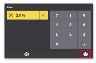
**Step 14**: Enter the desired long slope value and press tick mark icon (OK).
