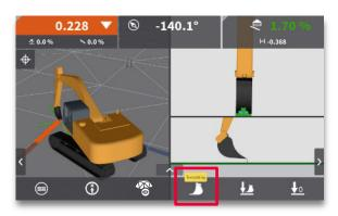
• Current bucket is shown in run-screen. Bucket name is displayed above the bucket icon in the quick access bar.
