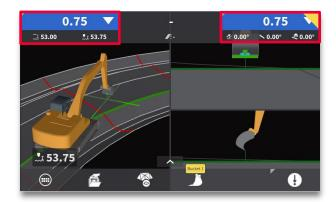
• The new surface will be represented by a bold green line. Cut/fill will be provided to this reference and design cross-slope and long slope will update to reflect the height reference selected.
