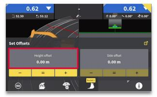
**Step 3:** Press the grey "Height offset" box for specific offset value input.
