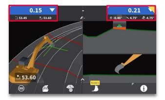
The selected reference will be represented by a bold green line. Cut/fill will be provided to this reference and design cross-slope and long slope will update to reflect the height reference selected.
