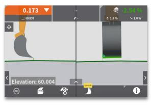
**Step 2:** Use "up/down" and "left/right" keys to place both "height" and "side" tool points at the control point position.
