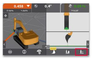
**Step 2:** Ensure tool point matches bucket position on the reference. Press the "bench 0" icon.
