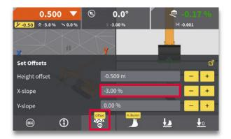
**Step 4:** Verify applied slope values. Press the model options menu to return to run-screen.
