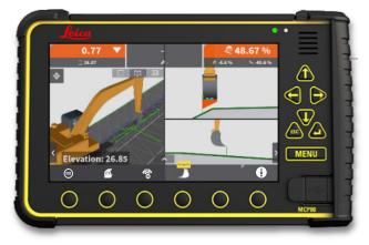
**Step 1:** Verify height tool point position. Height tool points are represented by a green icon on the blade (Left height tool point is shown).
