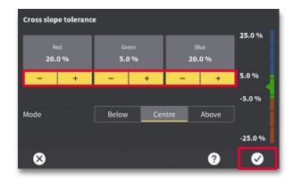
**Step 4**: Use the +/- buttons to increase or decrease tolerance for each field (**fill**, **on grade** and **cut**). Press tick mark icon (OK).
