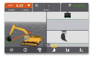
**Step 5:** Place the bucket above desired slope.
