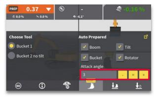
**Step 3:** Adjust "Attack angle" (if desired) by using the +/- keys or pressing the value field.
