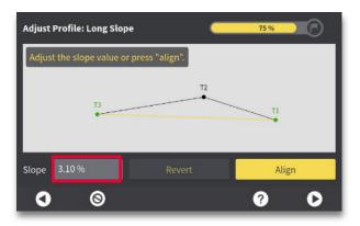
**Step 13:** Adjust the long slope per your project specifications by tapping the slope window.
