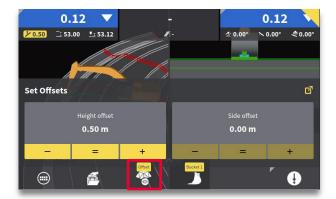
**Step 5:** The offset value will be shown as a yellow box in the upper left corner. Press the offset menu icon to return to run screen.
