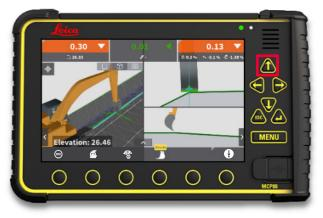
**Step 2:** Press **up** hard key to toggle side tool point to middle position.
