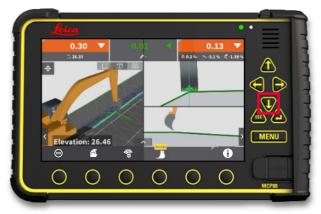
**Step 4:** Press **down** hard key to toggle side tool point in opposite direction.
