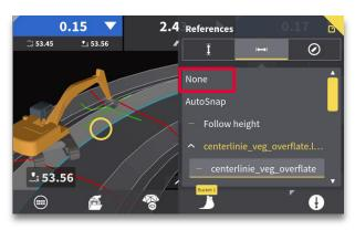
To clear the side reference, press and hold on run screen, press the icon, and select "None" to clear the side reference line.
