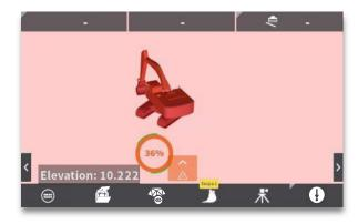
• The MC1 run screen displays the rotation progress.
