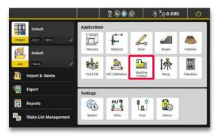
**Step 1:** Press the "Machine Control" application.
