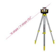
**Step 1:** Enter <u>both X-slope and Y-slope values</u> into the laser. Slope values entered into the laser MUST be the same as those entered into the panel.
