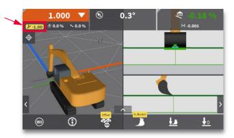
Cut/fill values are provided to the offset, and applied height offset is displayed in the secondary value bar. The offset surface is also illustrated in the cross/long section views.
