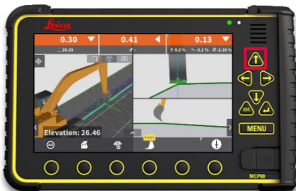
**Step 3:** Press **up** hard key to toggle side tool point to right tip position.
