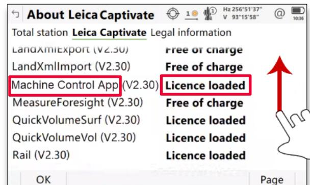
**Step 4:** Scroll the page upward until you see "Machine Control App". Verify that a license has been loaded.
