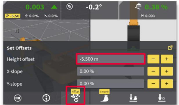
**Step 5:** Verify applied offset value. Press the model options menu to return to run-screen.
