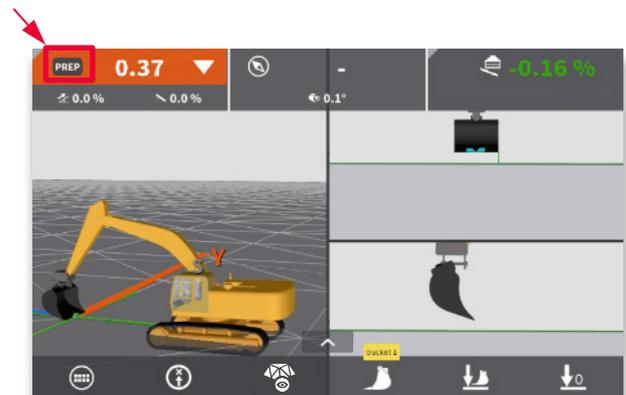
**Step 4:** Press the "PREP" button to activate CoPilot prepared mode (can be configured to an external button).
