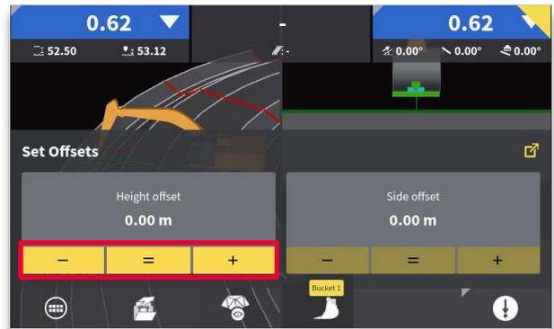
**Step 2:** Press - or + to offset your design by increments. Press = to set offset to current tool point height.
