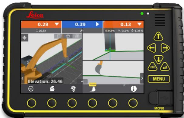
**Step 1:** Verify side tool point position. Side tool points are represented by a "teal" icon on the blade (Left side tool point is shown).
