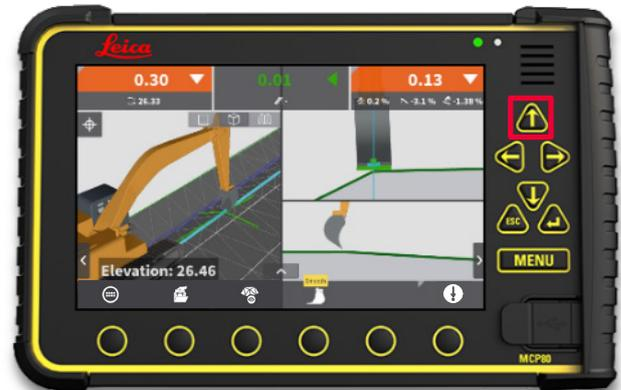
**Step 2:** Press **up** hard key to toggle side tool point to middle position.
