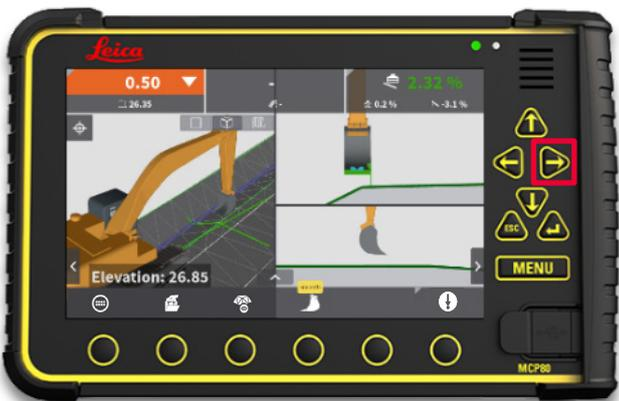
**Step 3:** Press **right** hard key to toggle height tool point to right tip position.
