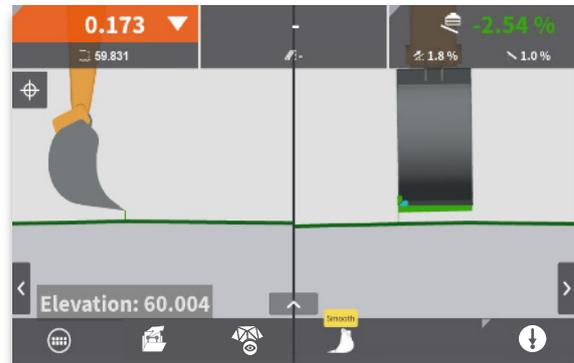
**Step 2:** Use "up/down" and "left/right" keys to place both "height" and "side" tool points at the control point position.
