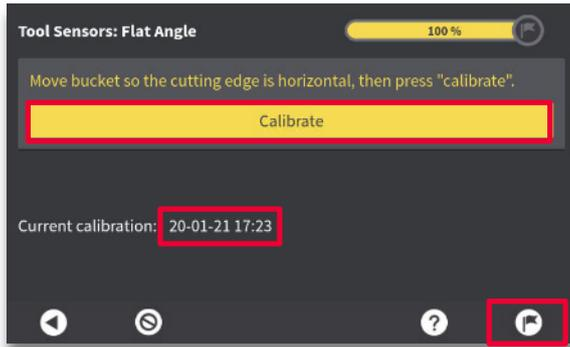
**Step 17:** Press "Calibrate". Calibration date/time is recorded for future reference. Press flag icon.
