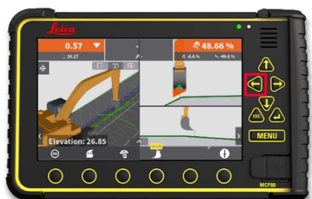
**Step 4:** Press **left** hard key to toggle height tool point in opposite direction.
