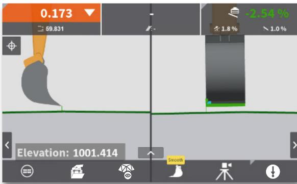
**Step 3:** Use "up/down" and "left/right" keys to place both "height" and "side" tool points at the control point position.
