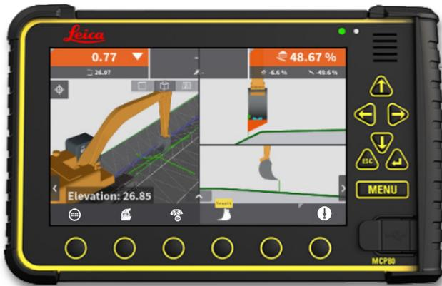
**Step 1:** Verify height tool point position. Height tool points are represented by a green icon on the blade (Left height tool point is shown).
