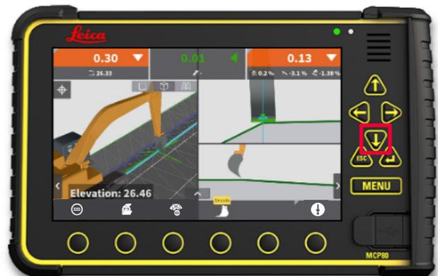
**Step 4:** Press **down** hard key to toggle side tool point in opposite direction.
