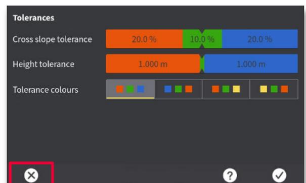
**Step 6:** Use the +/- buttons to increase or decrease the tolerance for each field (fill, on grade and cut). Press X (exit).
