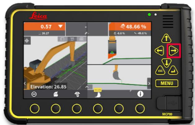
**Step 2:** Press **right** hard key to toggle height tool point to middle position.
