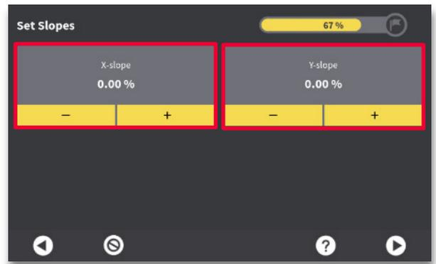
**Step 7:** Set X-slope and Y-slope to desired values.
