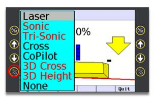
**Step 2:** Press "left side" configure softkey, and select **Laser.**
