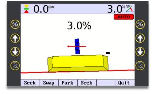
**Step 5:** Select A/M softkey on cross slope side to enable automatics. When "on grade", the arrows will NOT appear, and centre line of laser catcher illuminates green. Auto switch function has 4 options, selectable by tech.
