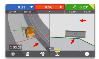
Press "up/down" hard key to toggle current tool point. Notice the offset distance changes relative to this point.
