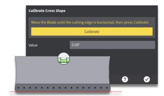
**Step 4:** Position blade horizontal using a digital level. Then press "Calibrate".
