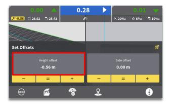
**Step 3:** Select grey "Height offset" box for specific offset value input.
