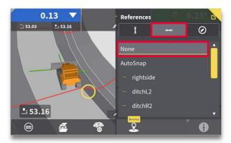
To clear the side reference, press and hold on run screen, press → icon and select "None" to clear the side reference line.
