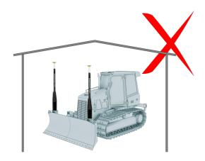
• GNSS Signal cannot be used indoors or under a canopy of trees.
