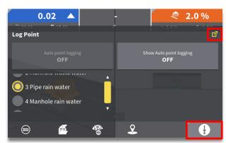
**Step 2:** Press and hold "Log point" button. Select a point code from available point code list and press "Log point" button to log a point with that point code. For more options select quick access button
