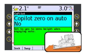
No = New reference angle is generated only when you press "Seek", or dial in desired long slope.
