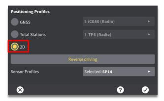
**Step 3:** Select "2D" positioning profile, and press "X" to return to run-screen.
