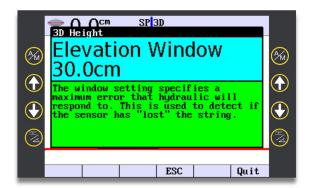
"3D Height Elevation Window" is set in the 2D UI > Configure > Adjust > Right 3x. If outside this window Auto will not engage. Suggested value is 30cm (0.98') typically set by technician.
