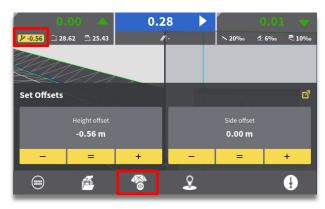
**Step 5:** Select "Offset" menu icon to return to run screen. The offset value is shown in the top left corner.
