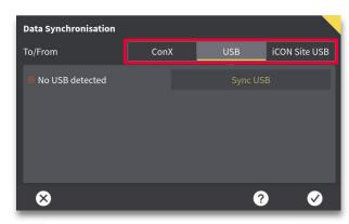
Selection of possible synchronisation methods. USB is only selectable when inserted.
