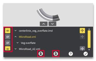
**Step 2:** Select the models that contain the references you want to make visible in the run screen. Press plus/minus icons to add or remove models in the command centre.
