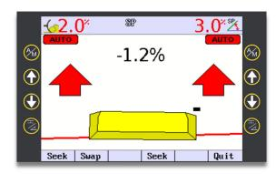
When auto is engaged, previously set long slope will be retained. CoPilot will NOT adjust long slope unless "up/down" softkeys are used to adjust values, or "Seek" is pressed to match current SP14 values.
