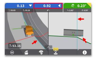
The offset distance, from current side tool point to selected line reference, is shown at top centre of the screen. A teal line represents selected line in run screen.
