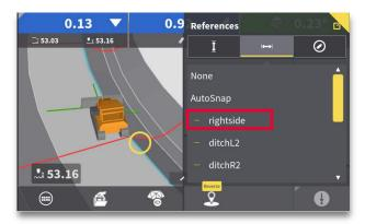
**Step 3:** Select desired line reference (line "rightside" shown here). The line closest to selected point is listed at the top.
