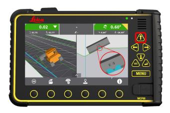
**Step 1:** Press "up" hard key to toggle side tool point to middle position.
