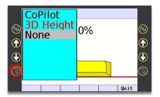
**Step 2:** Select "left side" configure softkey and use up/down arrows to select "None" for the Left tip configuration.
