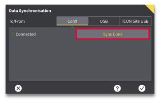
**Step 2:** Select desired synchronisation method. ConX is connected and therefore available for Sync.
