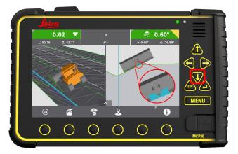
**Step 3:** Press "down" hard key to toggle side tool point in opposite direction.
