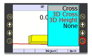
**Step 3:** Select "right side" configure softkey and use up/down arrows (Softkey or Keypad) to select "Cross".
