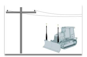
• When operating near "high power" lines, positioning quality could be affected.
