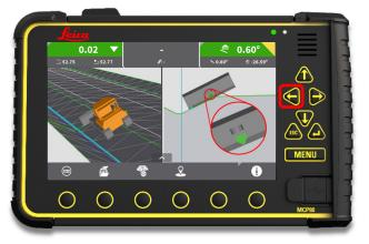
**Step 3:** Press "left" hard key to toggle height tool point in opposite direction.
