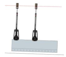
**Step 4:** Place blade on desired cross slope. Move laser receiver until green "on grade" indicators show. Alternatively, if using power masts, use "Seek" softkeys in + direction.
