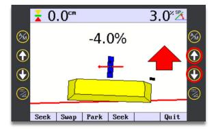
**Step 4:** Use "up/down" softkeys to dial in desired cross slope matching laser value. An arrow indicates the direction the cross slope controlled tip should move to be on grade.
