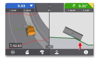
In this picture the blade is very close to match the slope value and height under "height tool point". However not an ideal work setup for the machine since most of the blade is on a different slope.
