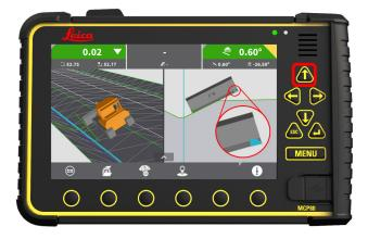
**Step 2:** Press "up" hard key to toggle side tool point to right tip position.
