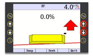
**Step 4:** Use right side "up/down" softkeys, to dial in desired slope. An arrow will indicate the direction the blade needs to move to match the slope.
