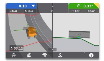
The new surface will be represented by a bold green line. Cut/fill will be provided to this reference and design cross-slope and long slope will update to reflect the height reference selected.
