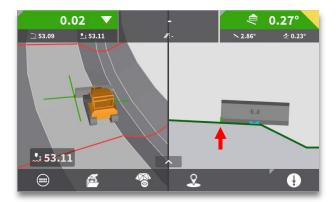
Blade shown in correct position to grade surface under current height tool point.
