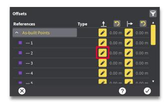
**Step 3:** Press the "Edit" button next to a reference to set an offset (height offset for point number 2 highlighted here).
