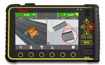
**Step 2:** Press "right" hard key to toggle height tool point to right tip position.
