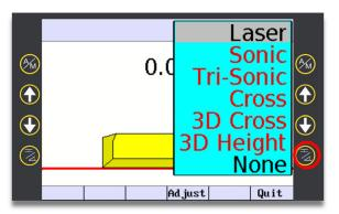
**Step 2:** Press "right side" configure softkey, and use up/down arrows (Softkey or Keypad) to select "Laser".
