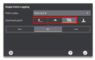
Step 3: Choose which tool point to use when logging a point (Current height tool point, current side tool point or specific tool point not used for height or side references). Select "X" to return to run screen.
