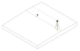
**Step 2:** If the grade has a dual slope, have the surveyor set hubs along X and Y axis.
