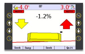
When auto is engaged, CoPilot will match long slope of the blade in its current position. If a different long slope percentage is desired, use "up/down softkeys to adjust while in auto.
