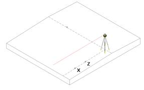
One hub along X axis will be used for "height benchmark" the other for cross slope (Adjust laser based on this X-slope).
