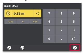
**Step 4:** Use keypad to input a value, and toggle the sign. A list of the last 3 height offset values are also listed for quick selection. Select check mark icon to accept value.
