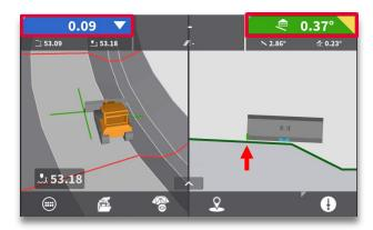
Cut/fill and slope values are based on the surface below current height tool point (Left height tool point shown).
