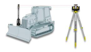
**Step 2:** Adjust height of your laser beacon and laser sensor:
