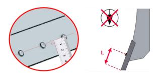
**Step 2:** Measure flat against surface of cutting edge to centre of bolt holes. This value represents your current blade wear.
