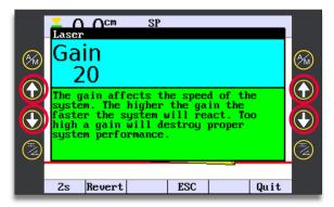
**Step 4:** Use up/down soft or hard keys to adjust gain value until hydraulics perform to satisfaction.
