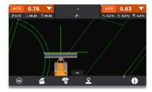
If the blade is raised outside of the configured elevation window, the system will go into red (inactive auto)
