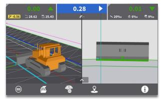
Cut/fill values will be shown, providing guidance to new height offset. Original grade will still be shown in x-section with applied offset.
