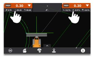
**Step 1:** Press and hold cut/fill on each side to get PREP to appear (This step is not necessary if set to A/M Mode: Toggle).
