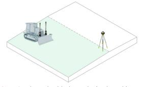
**Step 3:** Place the blade at desired working height. Adjust the laser receiver on your machine to catch the laser strike, at the center. Now, grade on the slope that matches the laser.
