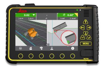
Height tool points are represented by a "green" icon on the blade (Left height tool point is shown).
