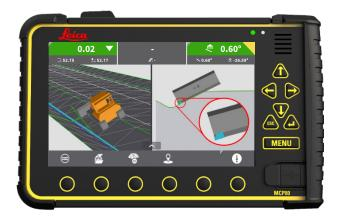
Side tool points are represented by a "teal" icon on the blade (Left side tool point is shown).
