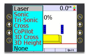
**Step 3:** Select "left side" configure softkey, and use up/down arrows (Softkey or Keypad) to select "Laser".
