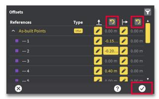
The "revert" buttons at the top can be pressed to remove offset values for all references. Press check mark icon (OK).
