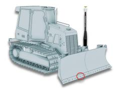
**Step 1:** Select a representative area of the cutting edge to measure blade wear (Avoid the outer .05m of the blade).
