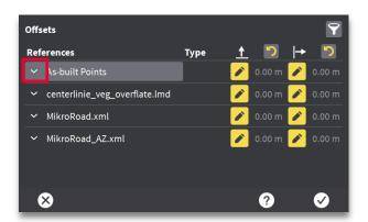
Here you have a list of all the referential models. By pressing the expansion arrow, a height and/or side offset can be applied to individual references.
