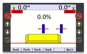
**Step 5:** Press A/M softkey, on either sides, to enable "Automatics". When "on grade" the arrows will not appear, and centre line of laser catcher illuminates green. Auto switch function has 4 options, selectable by tech.
