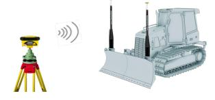
When using GNSS, your machine must be within radio range of the local base.
