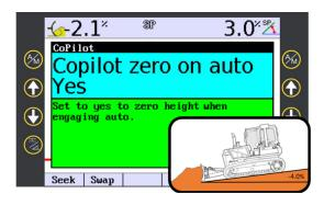
Yes = Every time you press "auto" button, a new CoPilot long slope reference surface is generated, based on blade position at that moment.
