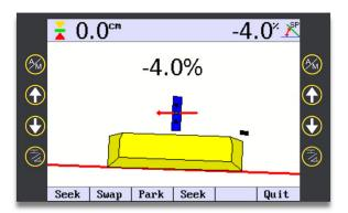
When laser receiver is within laser strike, a red horizontal arrow appears on screen.
