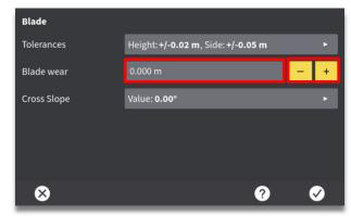
**Step 4:** Use + or - keys to increment blade wear value, or select the number to input manually.
