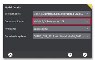
**Step 4:** Press the "Command center" menu, to access available models. You can also access the command center from the run screen (Workflow 03.)
