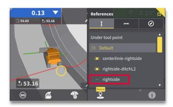
**Step 3:** Select the desired height reference (line "rightside" shown here). The line closest to selected point is listed at the top.
