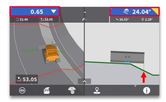
When design slope changes under current height tool point, cut/fill and slope values also change (Right height tool point shown).
