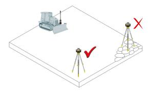
Stable ground, so the tripod won't shift or settle (Ground Vibration can affect operation of the laser).
