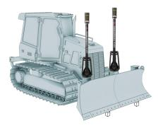
X-axis hubs can be used to establish cross slope manually, as pictured here.
