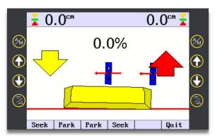
When laser receivers are within laser strike a red horizontal arrow appears on screen.
