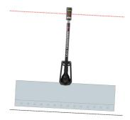
**Step 3:** Place blade on desired cross slope. Move laser receiver until green "on grade" indicators show. Alternatively, if using power masts, use "Seek" softkeys in + direction.
