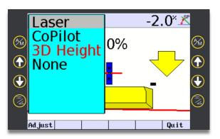
**Step 2:** Select "Configure" button and highlight desired sensor to adjust.
