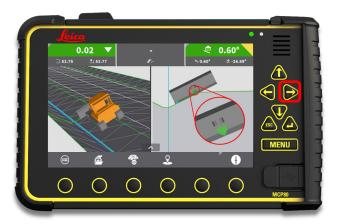
**Step 1:** Press "right" hard key to toggle height tool point to middle position.
