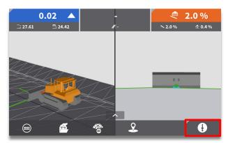
**Step 1:** Select "Log point" button to quickly log a point.
