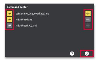
**Step 5:** Set which references that should be visible and available for selection in the run screen. Press the tick mark icon (OK) to return to previous menu.
