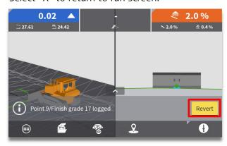
**Step 5:** If necessary, select "Revert" to remove previously logged point.
