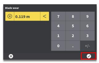
**Step 5:** Use keypad to enter blade wear value manually. Press "OK" to accept.
