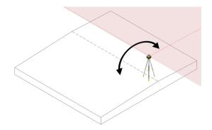
If the slope is mirrored, and if grading will be done on both sides, it is helpful to place your laser on the crown (This way the grade can be swapped on the laser without additional setup).
