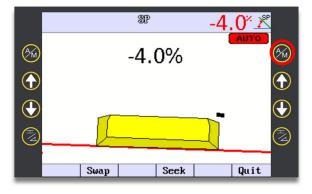
**Step 6:** Select A/M to engage automatic hydraulic functions (If equipped) and the blade will move to the desired slope.
