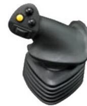
**Step 2:** Press installed "auto" button, to engage automatic control of the blade.
