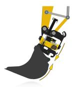
4. Raise the tiltrotator very slightly above the ground so that the tool moves towards the quick hitch.
