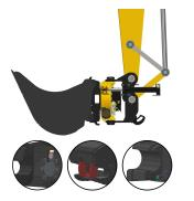
2. Check that the quick hitch lock's lock function has engaged:
