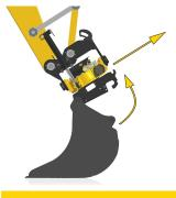
2. The locking bolts are now in the open position and the tool is free. Carefully raise the tiltrotator from the tool.
