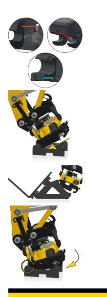
1. In the case of Q-Safe, check that the orange indicator rod is out.
